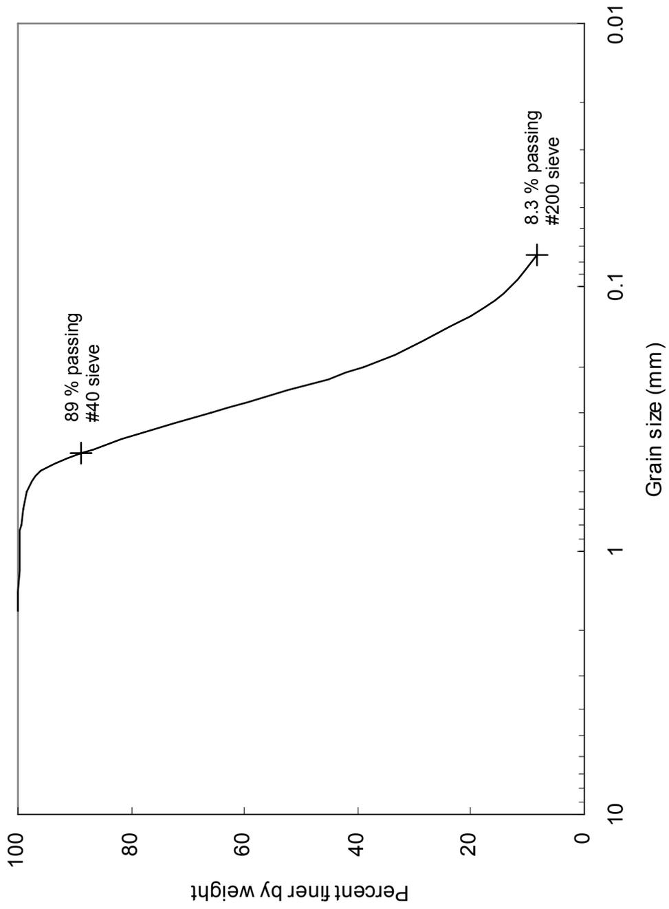
Figure 4: Grain size distribution of the fine, red, clayey sand – *Soil B* (after James et al., 1985)
