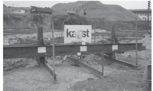
Figure 4. Test pile's construction
